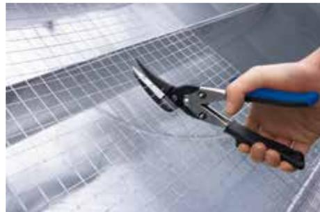
**Shape and straight cutting snips, robust D17ASS**
